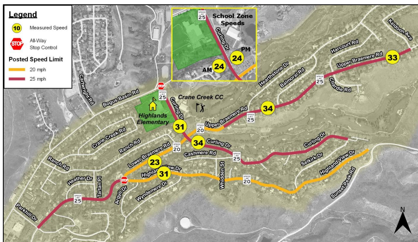
Figure 2-3. 85 th percentile speeds before mitigation measures
